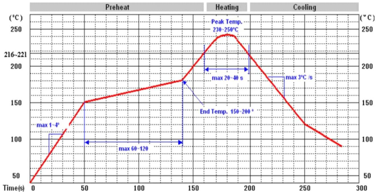
**Note:** The final soldering temperature chosen at the factory depends on additional external factors like choice of soldering paste, size, thickness and properties of the baseboard, etc. Exceeding the maximum soldering temperature in the recommended soldering profile may permanently damage the module.
